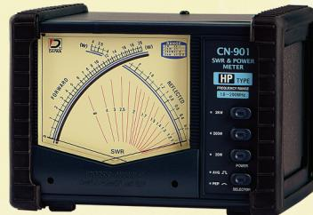
SWR and Power indicators are installed in one meter unit. One scale will be indicated at the crossing point of the 2 needles. This unique feature makes it possible to read all of Forward Power, Reflected Power and SWR at the same. HP type can also measure P.E.P Peak Power in SSB operation.(can not measure Reflected Power range.)
