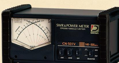
SWR and Power indicators are installed in one meter unit. One scale will be indicated at the crossing point of the 2 needles. This unique feature makes it possible to read all of Forward Power, Reflected Power and SWR at the same time.
