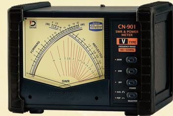
SWR and Power indicators are installed in one meter unit. One scale will be indicated at the crossing point of the 2 needles. This unique feature makes it possible to read all of Forward Power, Reflected Power and SWR at the same time.
