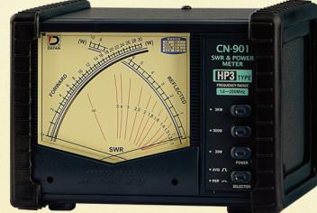
SWR and Power indicators are installed in one meter unit. One scale will be indicated at the crossing point of the 2 needles. This unique feature makes it possible to read all of Forward Power, Reflected Power and SWR at the same. HP type can also measure P.E.P Peak Power in SSB operation.(can not measure Reflected Power range.)
